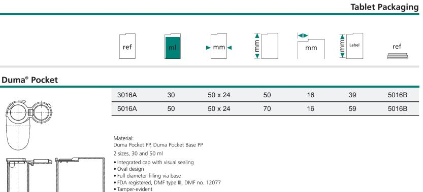
Produced by injection moulding
